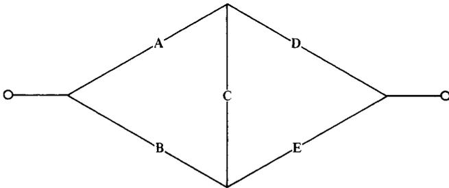
**Figure 6.** Bridge circuit.
