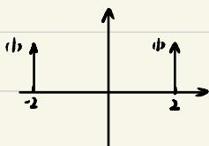
$$\begin{aligned} f(t) &= f_1(t) * f_2(t) = f_1(t) * (\delta(t+2) + \delta(t-2)) \\ &= f(t+2) + f(t-2) \end{aligned}$$
