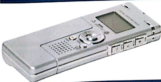
Some digital recorders have built-in USB connectors to make it easy to download files to the computer.
